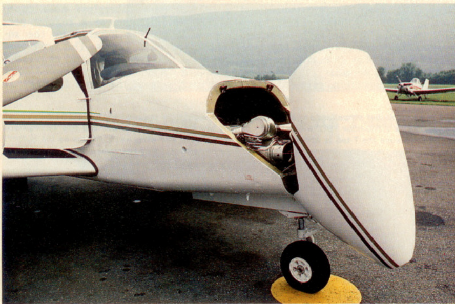
A fold-down fiberglass nose cone makes some of the Seminole's systems readily accessible.
